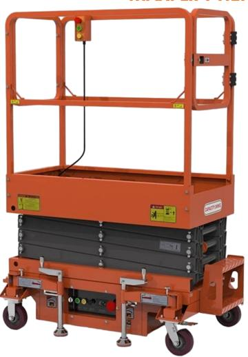
Mobile aerial work platforms are much more versatile than mobile towers, thanks in part to their one-touch height adjustment.
