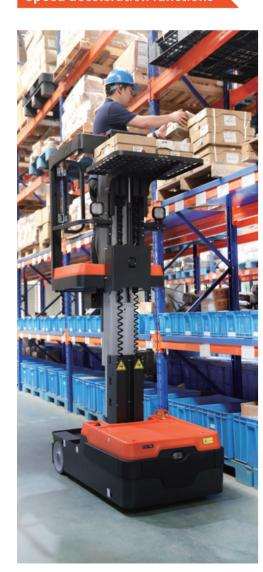
While platform is raising to its maximum height, the maximum available lift and drive speeds will go through three steps of speed settings according to the following lift height ranges for the platform: 0-500mm, 500-1500mm, 1500-3000mm to ensure the truck's stability and operator's safety.
