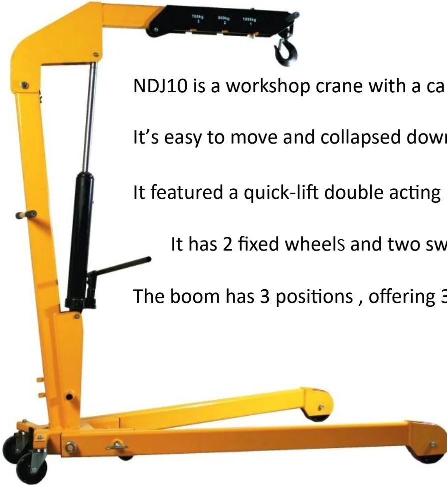
NDJ10 is a workshop crane with a capacity of 1000kg.
