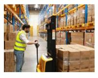
Easily maneuvered with the handle in the vertical position by pressing the turtle-speed button.
